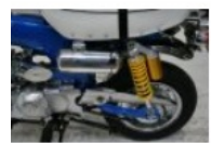
Exterior Fuel Tank (ZHX851)
